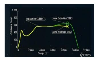
The Vinci engine ran up to about 18 minutes after liftoff, after which Ariane 6 demonstrated that it can reproduce the typical flight profile of the Ariane 5 ECA version.
